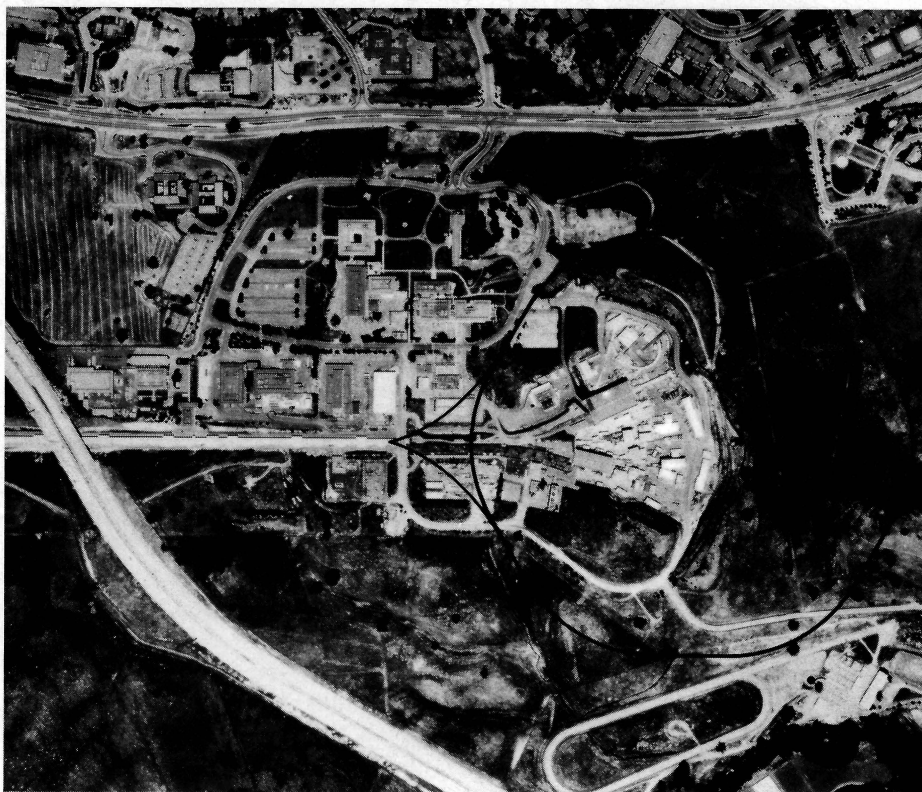
Location of the PEP 18 GeV electron-positron storage ring on the site at Stanford. The 22 GeV linac, coming in from the left will provide the particles for injection. The break-in to the switchyard for the injection tunnels will start in the Summer.
